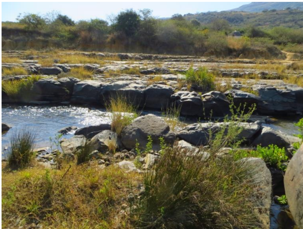
Figure 2-28 EWR Site BM2. Photograph of cross-section B, the bedrock chute for high flows, through which the cross-section was surveyed, taken from the right bank on 12 July 2014 (discharge of 0.27 \text{ m}^3/\text{s} ).
